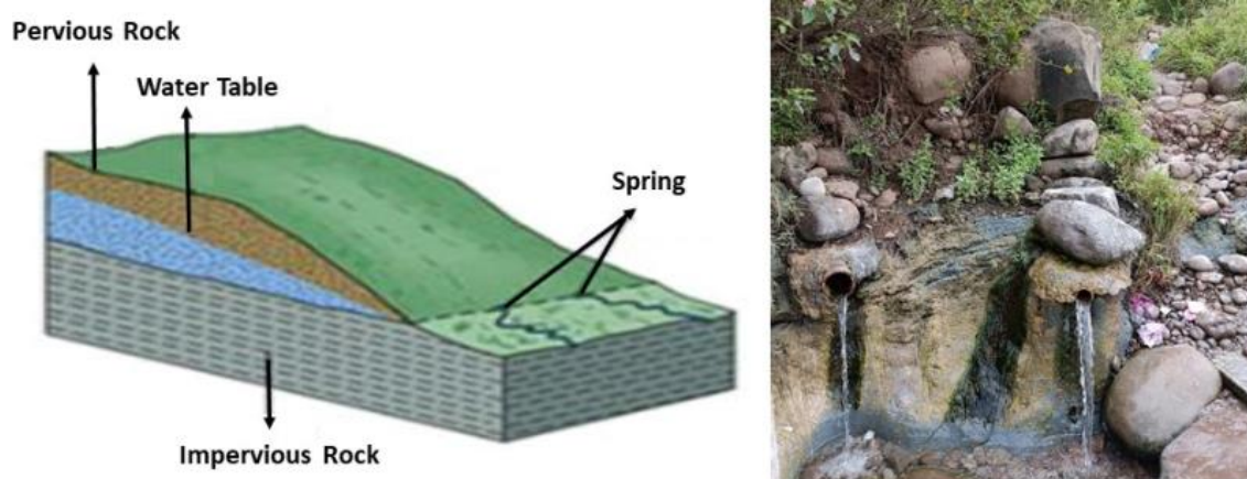
Fig. 4: Conceptual diagram of Contact Spring
