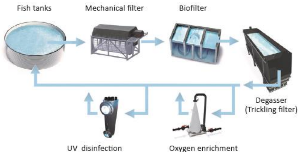
Fig. 1: Components of RAS
