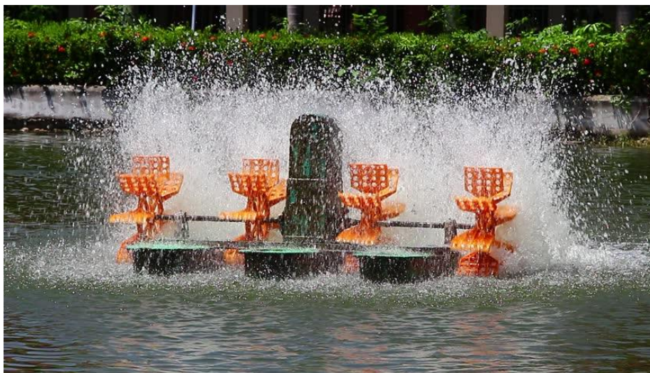
Figure-4 Paddlewheel type Aerator
